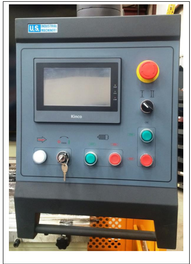
Photo above is "Simple CNC". This control is CODE ONLY, with touch screen input. This allows 2-axis programming of X (backgauge) and Y1 (ram position).
