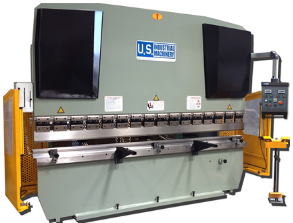
Photos above are MANUAL Hydraulic Press Brake with front-operated power backgauge, power ram adjustment, both with manual fine adjustment and digital readouts. Operators pendant has dwell adjustment for ram, key lockout, jog control and E-stop.
