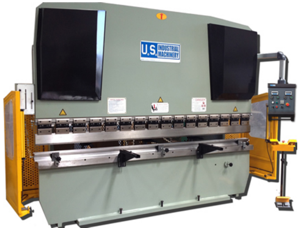
Photos above are MANUAL Hydraulic Press Brake with front-operated power backgauge, power ram adjustment, both with manual fine adjustment and digital readouts. Operators pendant has dwell adjustment for ram, key lockout, jog control and E-stop.
